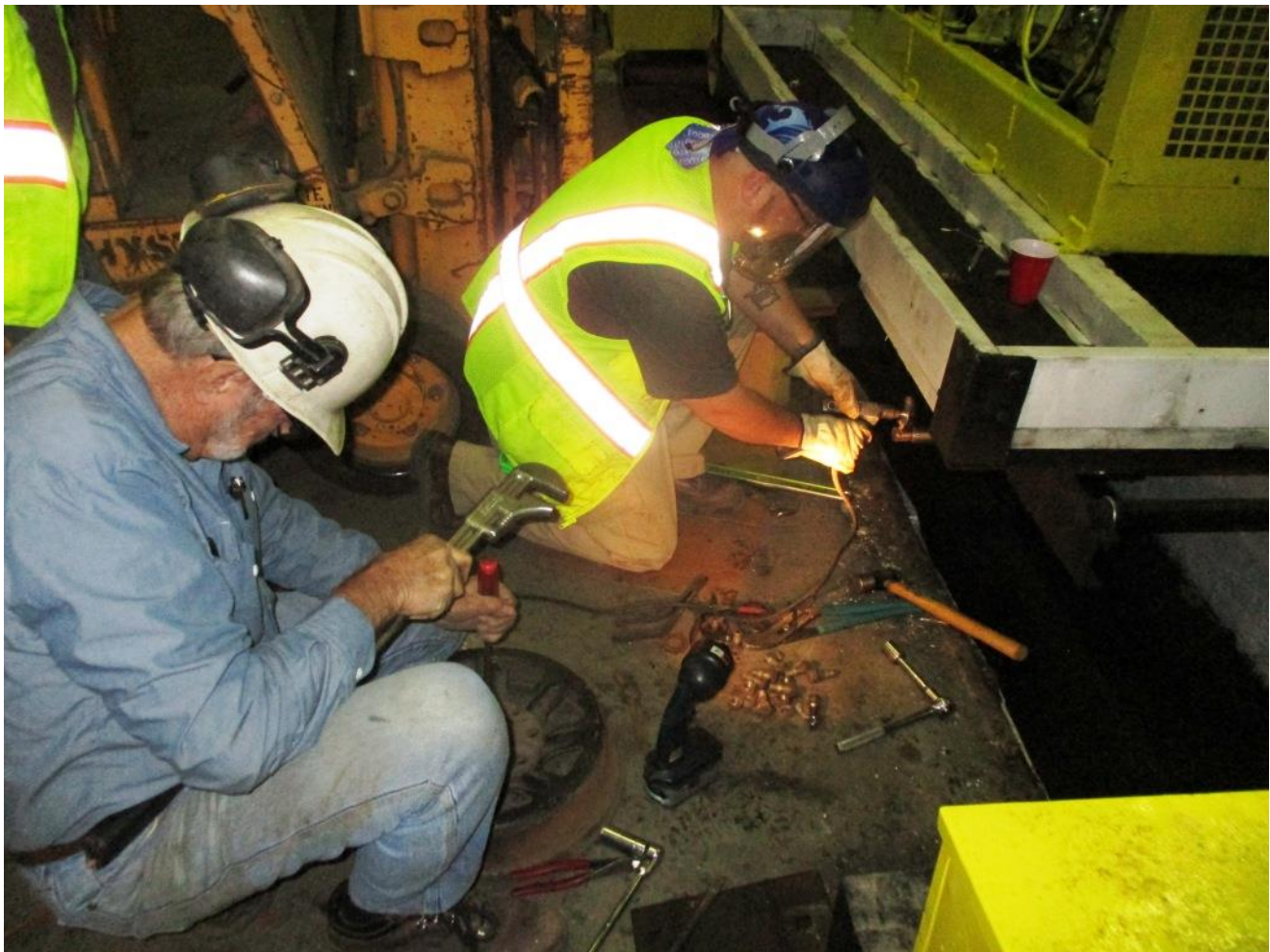
Alan and DJ replace the wonky wheel on the air-compressor's track-cart
