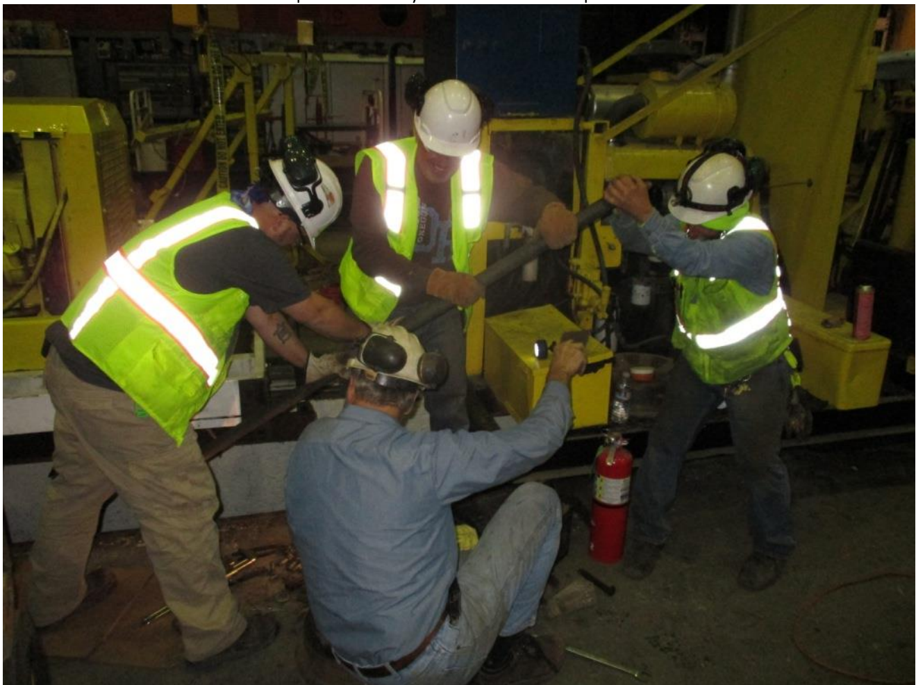
DJ, Dave W., and Joe combine forces to tighten-down the castellated nut on the air-compressor cart's wheel hub
